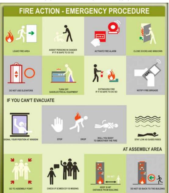
Fig. 5.14: Fire evacuation process
